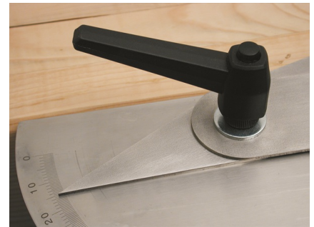
legs can be fixed by a large clamping lever
