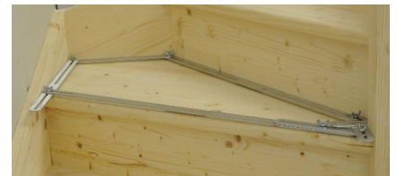
For transferring polygonal contours to workpieces
