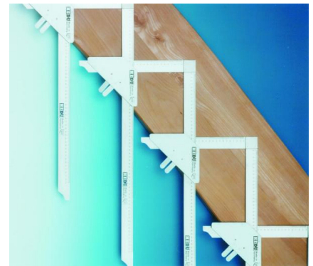
Ideal for marking the stringers of spiral staircases
