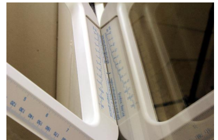
Measurement of glass thickness by reflection in the pane
