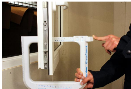
Thickness measurement of single and insulating glass
