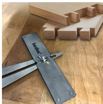
The tongue has a 1:8 inclination
