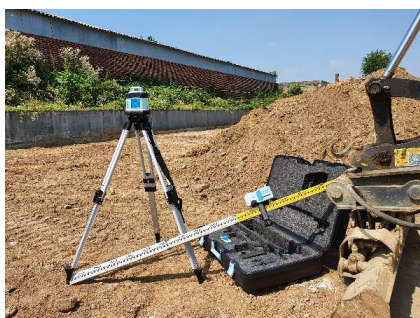
Complete set for leveling in a large case with tripod and measuring stick.
