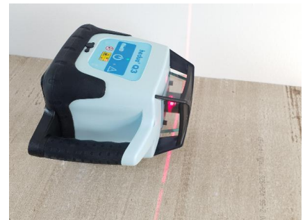
Horizontal and vertical self-levelling by servomotors up to 5° inclination.
