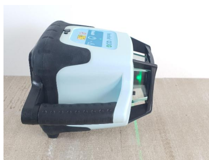
Horizontal and vertical self-levelling by servomotors up to 5° inclination.
