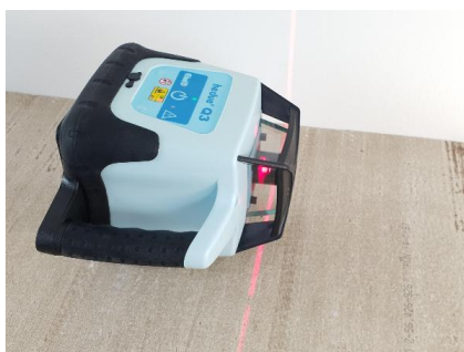
Horizontal and vertical self-levelling by servomotors up to 5° inclination.
