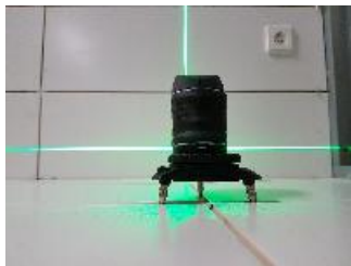
Better visualization of the laser line indoors due to the green laser diode.
