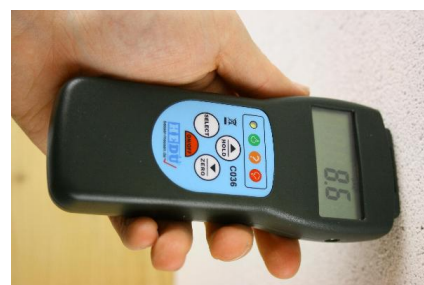
Determination of the moisture content of wood and building materials within seconds
