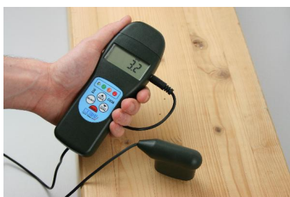
Suitable for wood and building materials between 200 and 3000 kg/m 3 .
