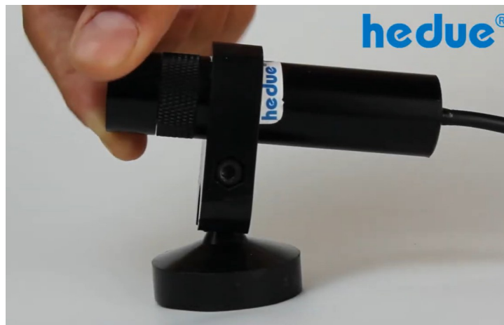
Fig. 3: Focusing by turning the knurled front part of the laser
