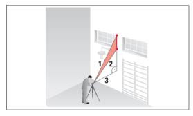
e.g. determining the height between point 1 and point 2 using three target points.
