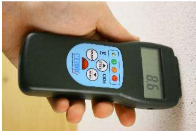
First remove the cap, then put the measuring area onto the material.
