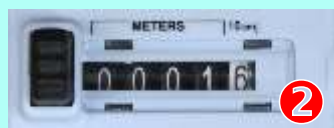
2 Measuring range up to 9.999,9 m Tolerance 0,08% Release 10 cm
