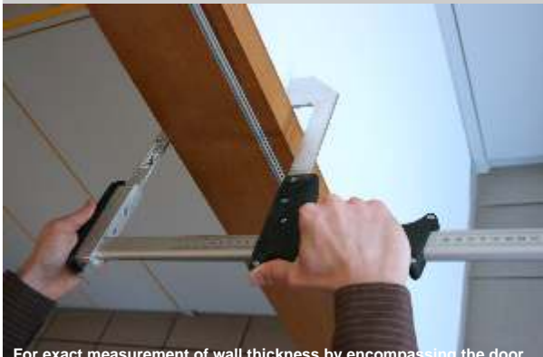
For exact measurement of wall thickness by encompassing the door.
