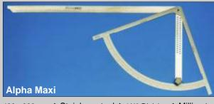
480 x 900 mm ◆ Stainless steel ◆ 1/4°-Division ◆ Millimetre scale on the scales and lace rip ◆ Durably etched scaling ◆ Big star knob
