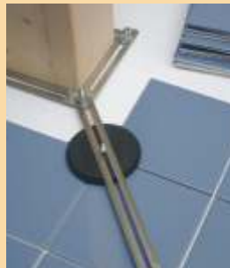
Angle template 180 x 180 mm with two extensions of 70 mm each
