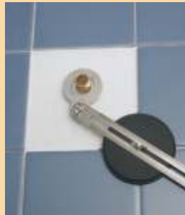
33 mm circular template for hole determination
