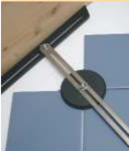
330 mm ruler guide for angle measurement
