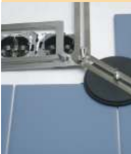
Rectangular hole template 64 x 100 mm (here fitted to the angle template)
