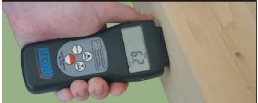
2 in 1: This moisture measuring instrument offers a needle-mode (picture above) and a non-destructive searcher-mode (picture below).
