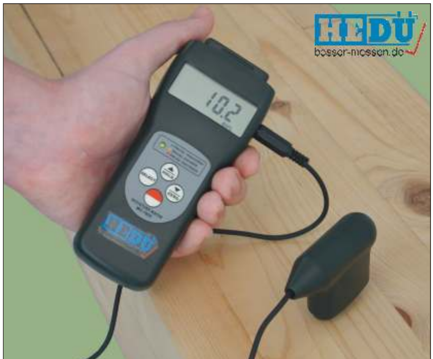
2 in 1: This moisture measuring instrument offers a needle-mode (picture above) and a non-destructive searcher-mode (picture below).
