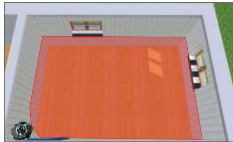
When you set up the laser in a corner of the room, nearly the whole room is covered by the laser line. For this job you can use a monopod or a wall tripod.
