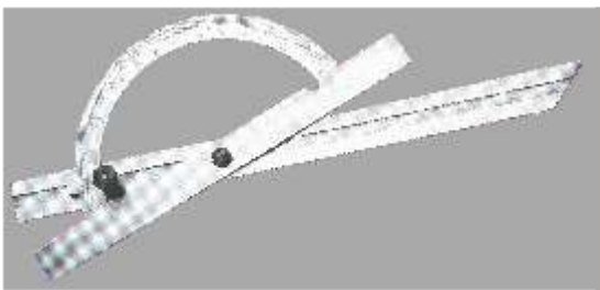
Measure of the inner corner (blue), and this angle will be halved (red) automatically
