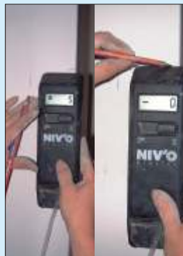
The difference to the zero level is displayed in mm. So the zero level is easy to transfer.
