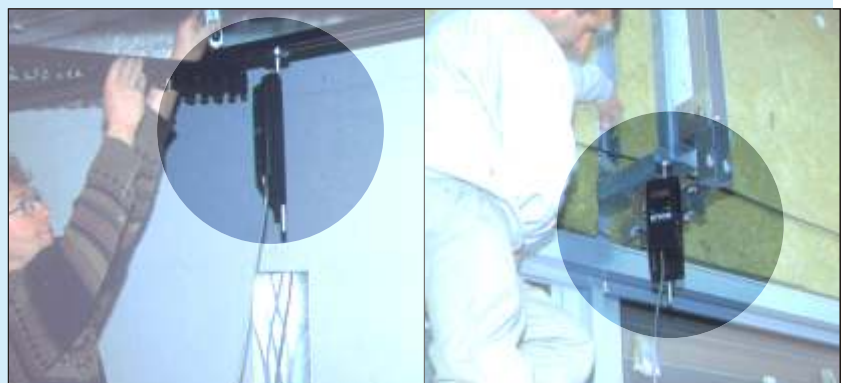
The H-set (incl. Magnet) is perfect for levelling hanging at the ceiling.
