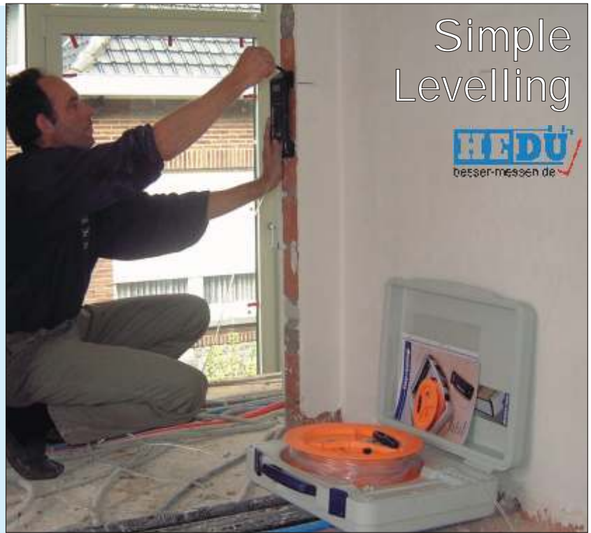
With the niv±comp levelling jobs can be done easy, by only one person. And the accuracy is 2mm on 48m.
