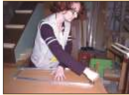
The transferring of the form is really easy by the angle template.
