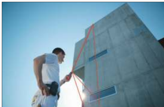
Indirect altitude measure of the high of a building will be done by the Pythagoras function.
